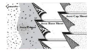
**GENERAL**. This specification is for use over any type of approved structural deck which is not nailable and which provides a suitable surface to receive the roof. Poured and precast concrete decks require priming with **Assa Asphalt Primer** prior to application of the first heat-welded modified bitumen ply.
